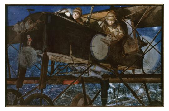
21. In 1918 the French used the Breguet 14 for day and night bombing. The bomb racks were designed by Michelin and the circular transparent panel on the side of the observer's cockpit was designed to help him aim the thirty-two 8 kg bombs which the aircraft carried. The Breguet 14 was used in large numbers on a number of fronts, was supplied to allies, including the Americans, and had a successful post-war career.
