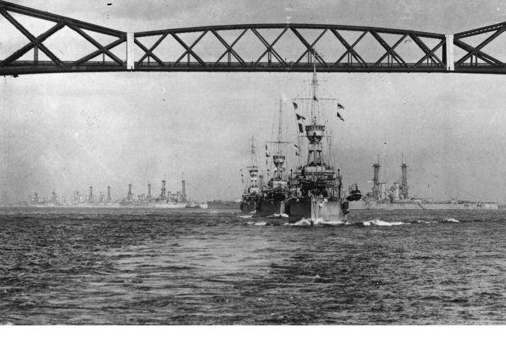
Three Arethusa class light cruisers, each with a Sopwith Camel on a flying-off platform over A-gun, passing under the Forth bridge. In the background, recognizable by their cage masts, are United States battleships serving with the Grand Fleet as the 6th Battle Squadron.
