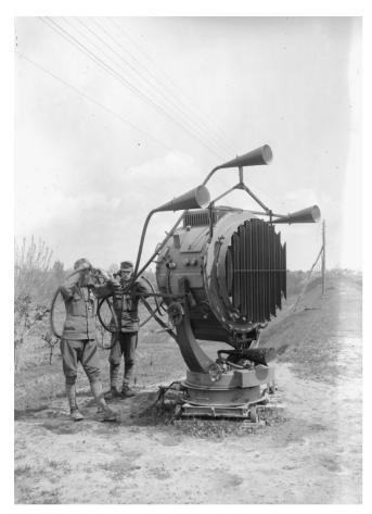
The war in the air prompted the development of additional technologies. Searchlights were required at night, both to detect enemy aircraft and to direct friendly ones. During the day, listening posts fulfilled similar functions. This combined apparatus is being used by Austro-Hungarian troops on the Italian front in May 1918.
