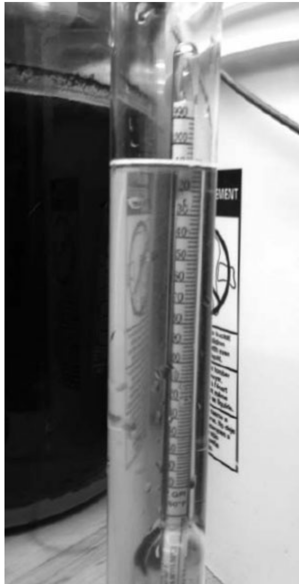
Fig 1.5: Measuring final gravity (note clarity).
