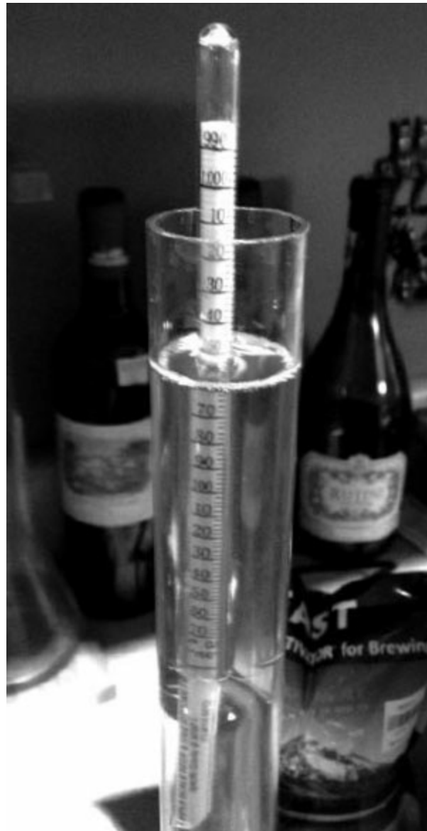
Fig 1.4: Measuring starting gravity.
